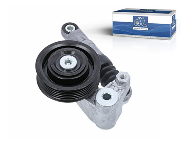
Belt tensioners guide and redirect the belt, ensure the correct tensioning of the V-belt or V-ribbed belt as well as the damping of belt vibrations resulting from changes in load of the motor or the auxiliary units. Furthermore, belt tensioners prevent the belt from severely vibrating where the tightening lengths are long (free, not overlying section of the belt). Belt tensioners and their components are heat-resistant and can withstand high mechanical loads.
