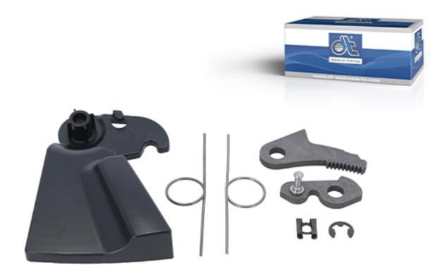
This item is a repair kit of the left seat, which is suitable for both left-hand drive and right-hand drive. It is used to vary the position of the backrest.
