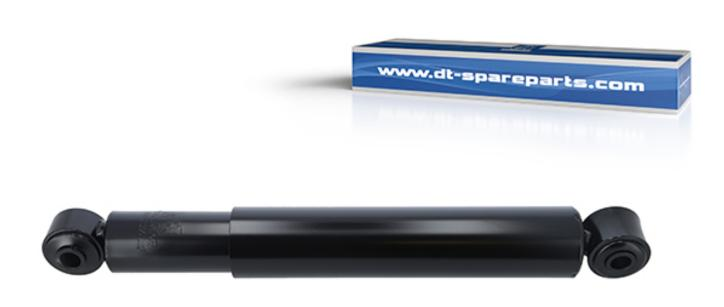
The shock absorber or vibration damper has the task of compensating for road irregularities and reducing or braking vibrations of the vehicle spring. Together with the spring, the shock absorber is the connection between the body and the wheel suspension.
