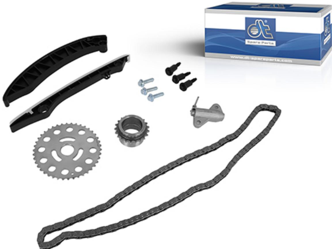
The timing chain is located at the front of the engine and is mounted on two sprockets – on the crankshaft and on the camshaft. The timing chain transmits the rotary motion of the crankshaft to the camshaft, which ensures that the valves open and close at the right time.
