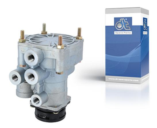
The trailer control valve in the towing vehicle causes the brake system of a trailer to be supplied with compressed air. It also controls the trailer brake system via the service brake system of the towing vehicle and via the parking and auxiliary brake valve.
