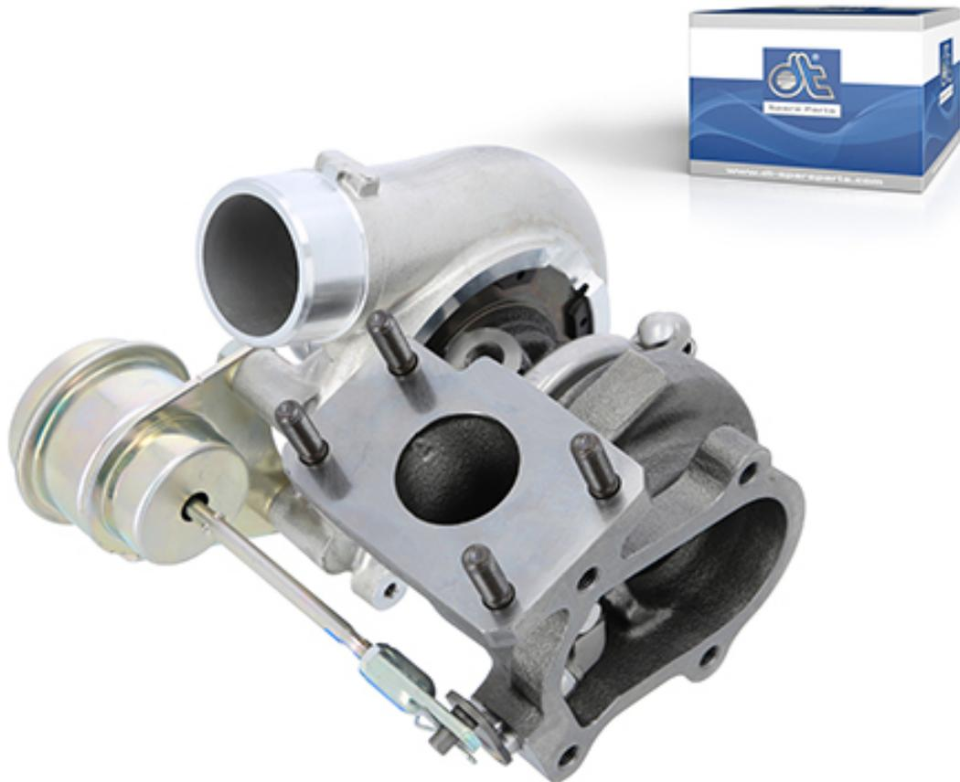
Exhaust turbochargers consist of two flow machines; one turbine and one compressor that are placed on a joint shaft. The compressor draws in fresh air, which is then pressed through the charging air cooler for cooling down and then at up to 2 bar in the combustion chamber.
